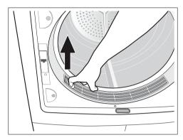
Push down the unlock button on the large mesh filter.
